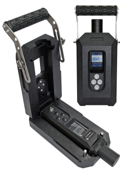
Neutron moderator for increasing sensitivity to neutron radiation
